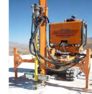
Self moving drilling unit with rubber tracks suited to execute vertical, horizontal or inclined holes, the power pack is equipped with a petrol motor (on request electric or gasoline). It is possible to install an hydraulic rotating head to utilize the pneumatic Down The Hole Hammer or rotation pneumatic or hydraulic rock drills to execute holes of various diameter.
